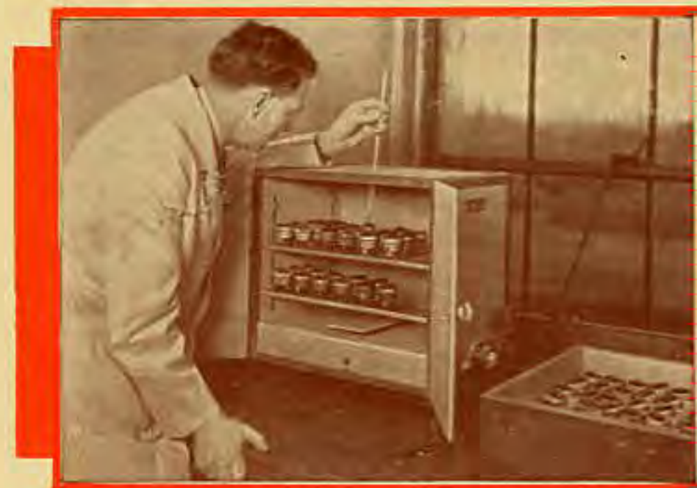
All transformers are first baked in this thermostatically controlled electric oven to remove every trace of moisture, then specially treated to prevent moisture afterwards affecting them.
