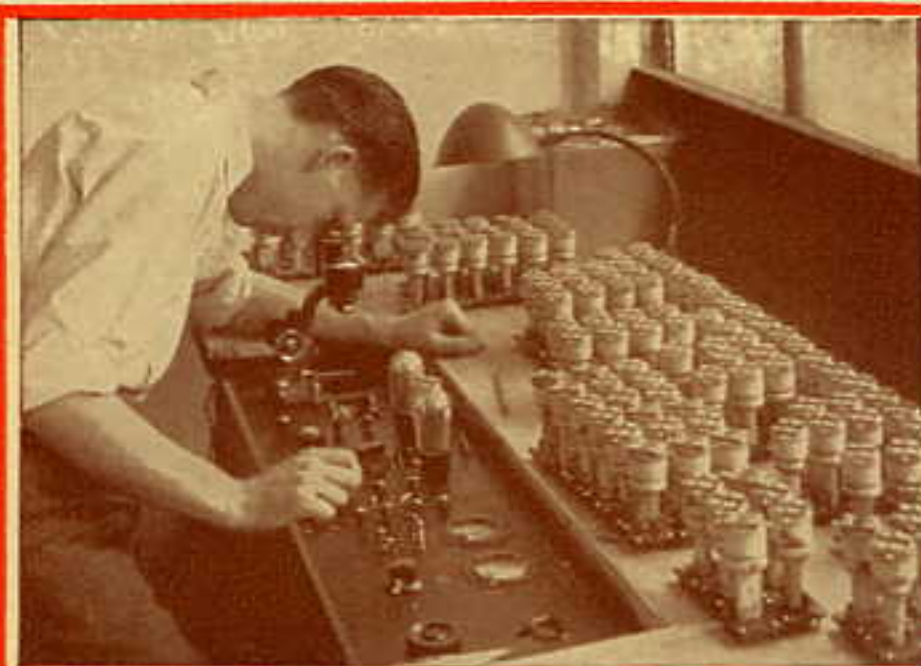
All I. F. Transformers are checked on the oscillator and vacuum tube voltmeter shown here. To insure accuracy, a high powered microscope is used to observe reading.
