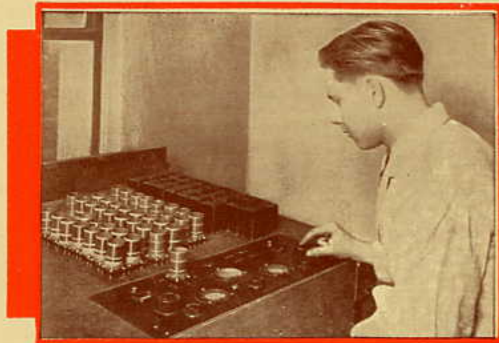
To insure the greatest efficiency in receivers, the oscillator and antenna coils must be matched to each other perfectly. This apparatus measures inductance of coils with 80 or 90 turns to within a third of a turn.
