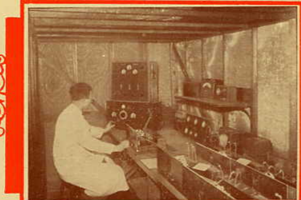
The finest and most modern radio measuring apparatus in the country is here used to make the final tests of completed receivers.
