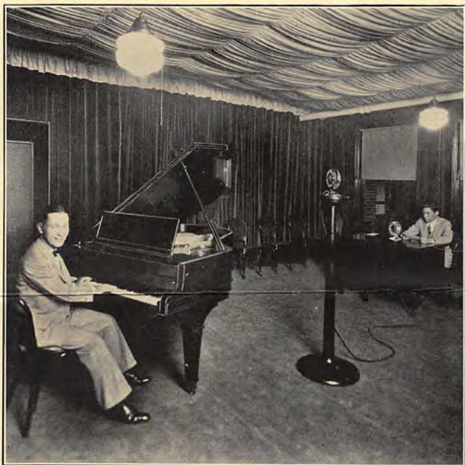
The Studio, Radio Station WJBL, with announcer Rickards at the control desk and Earl Voyles at the Baldwin grand piano. Two microphones are used, one for announcements, the other for programs. The picture shows the draperies and the ceiling canopy which make the room sound-proof.
