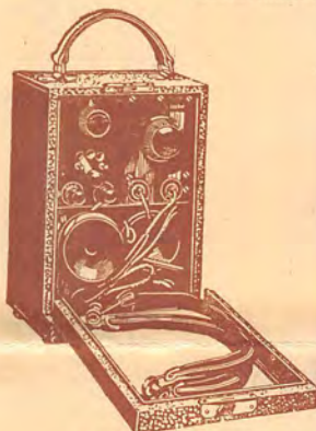
P-11—A one tube portable—the Camera of Radio—fits in the corner of hand bag, weighs only 4 3/4 lbs. complete.
