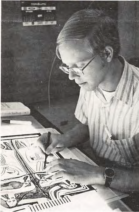
Laying out a printed circuit board
