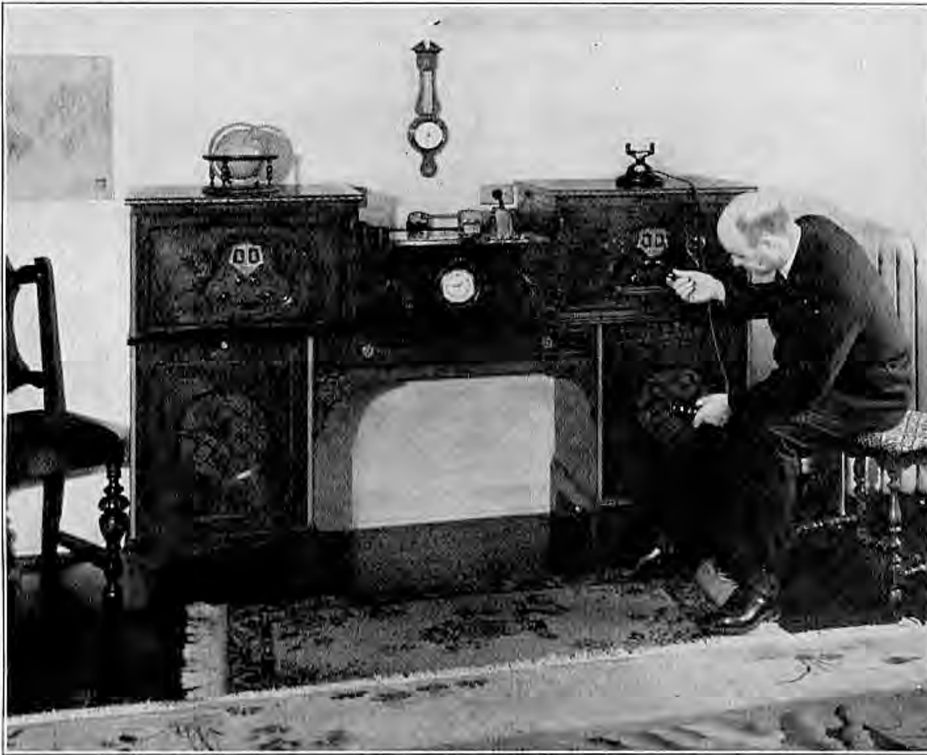
View Above Shows How Telephone Receiver Was Held in Front of Speaker to Send Signal Back to Australia
