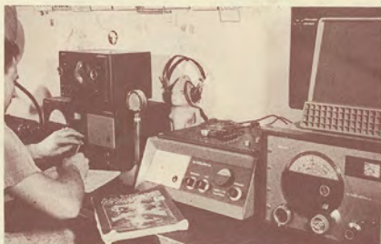
In the "Shack-on-Wheels," radio operator can pursue his work under difficult conditions of travelling over bad roads or tracks or open plains. During the war it was established that this Hallicrafters unit was able to maintain communications while running at 60 miles an hour over desert roads.
