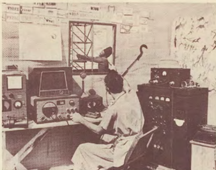
A model, built for testing purposes, of the base camp's permanent "Shack." Operator is directing a bay in adjusting one of the four directional antennae which will allow the station to blanket the entire globe.
