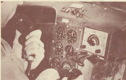
High up in the plastic bubble of the "Humming Bird" a member of the expedition can make his report to the base camp or synchronize the helicopter's flight with the movements of other units on the ground, by the use of the Hallicrafters Skyfone.
