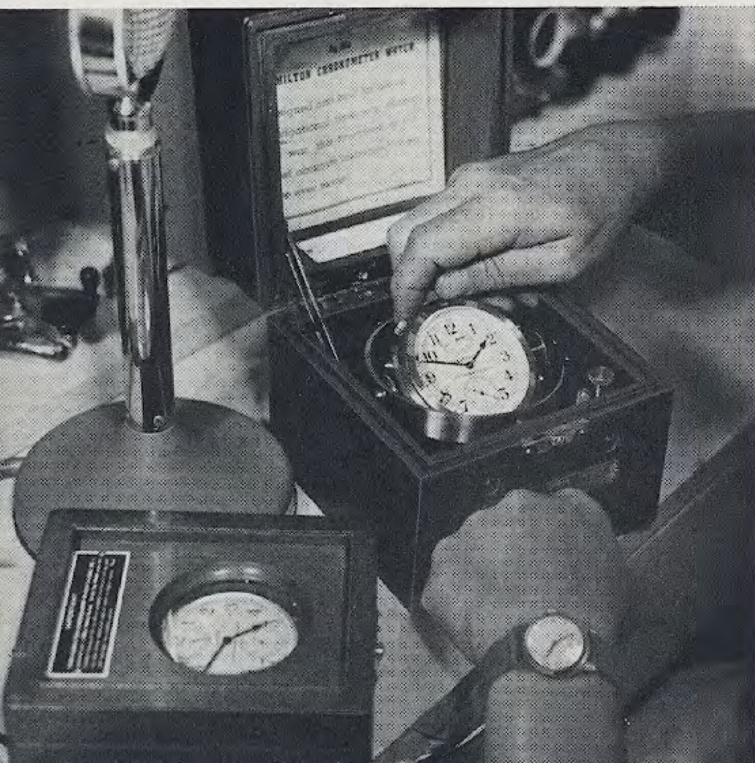
CHECKING EXACT TIME with Hamilton chronometers for precision in radio communications.
