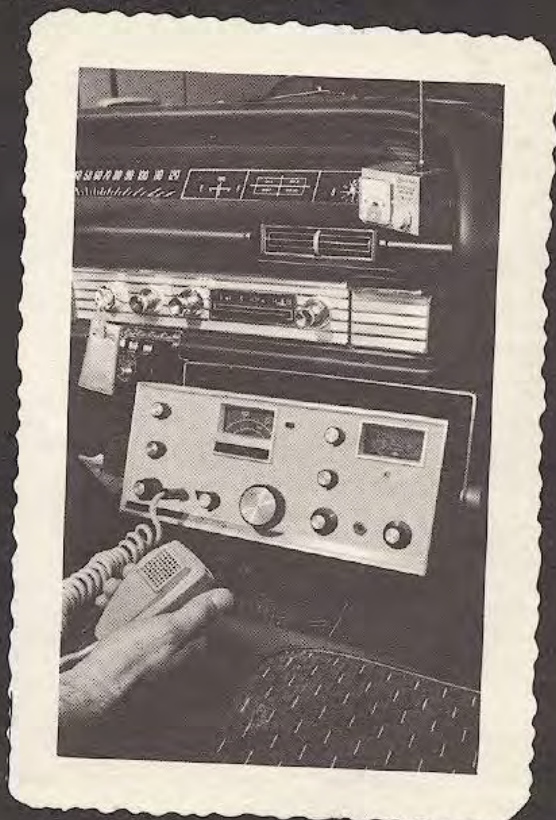
The NCX-3 SSB/AM/CW transceiver is a familiar sight in ham shacks and automobiles all over the world. The NCX-3 with its accessory AC or DC power supplies is a complete 200 watt 80, 40, or 20 meter amateur station.
