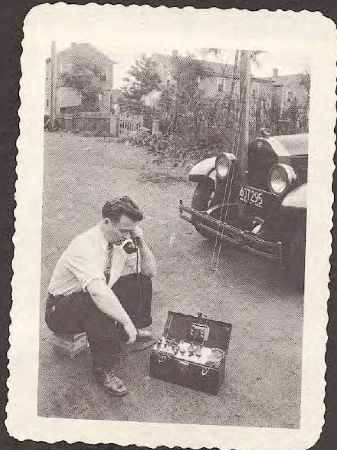
1933 -- The first amateur transceiver -- the 5 meter model TRW. Notice the light weight mobile antenna mounted on the bumper of the Buick.
