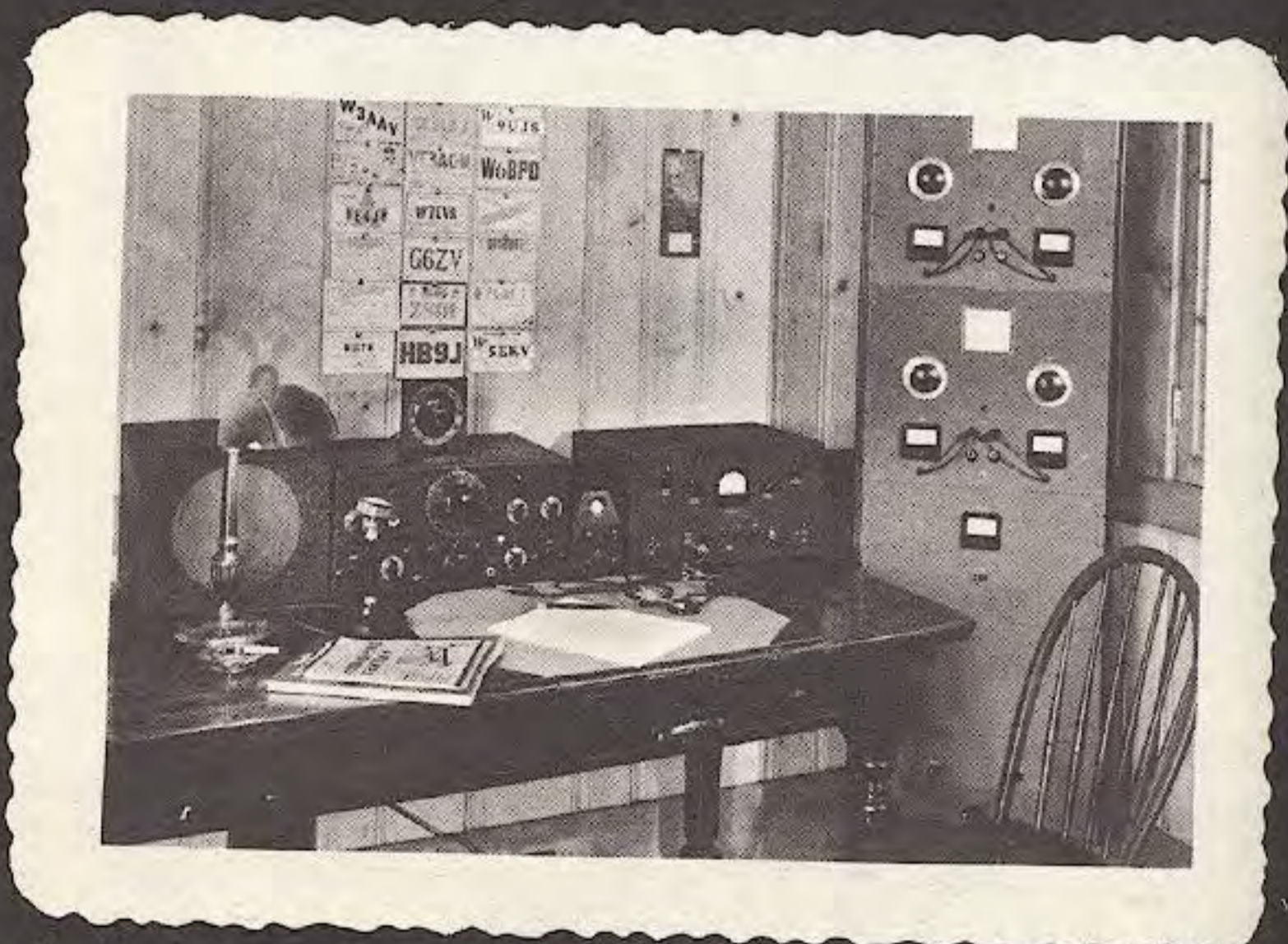
A deluxe amateur station of the late '30's -- NC-101X receiver, CRM 'scope, NTE exciter and the '600 transmitter.
