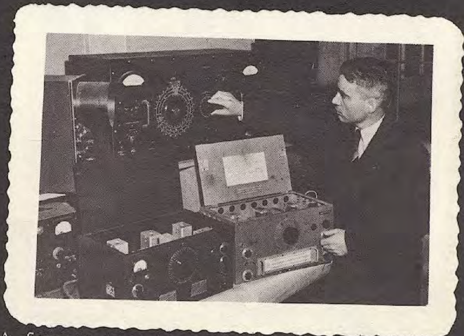
A famous war-time compliment to National -- the receiver on the right is an identical copy of the HRO manufactured by the Germans for their military communications.
