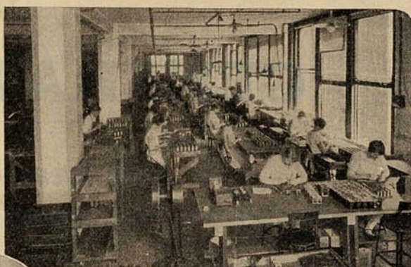
A transformer assembly department. Each transformer is given six tests, three under actual amplifier operating conditions.
