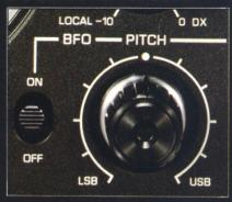
The beat frequency oscillator features exclusive independent detection circuitry which generates a carrier that demodulates SSB (single side band) and CW (continuous wave) signals. SSB includes amateur radio, CB, ship-to-shore and so on, while CW covers Morse communications. Models RF-2800 and RF-4800 have BFO with Pitch Control which is fully variable from upper to lower side band signals for optimum reception and clear demodulation of SSB and CW.
