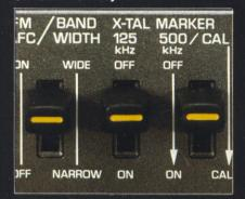
With the RF-2800 and RF-4800 calibration is performed by setting the dial at 10,000 kHz of 15,000 kHz for time signal transmissions (or any exact frequency known) and using the calibration knob. On these models, precision tuning can be achieved to 1 kHz. The RF-2200 uses Double Check Crystal Markers. One is a 500 kHz marker/calibrator, the other 125 kHz. Used together, you can calibrate and fine tune to within 10 kHz.
