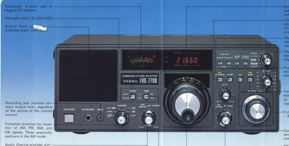
Built-in digital display provides for time and frequency indication.
