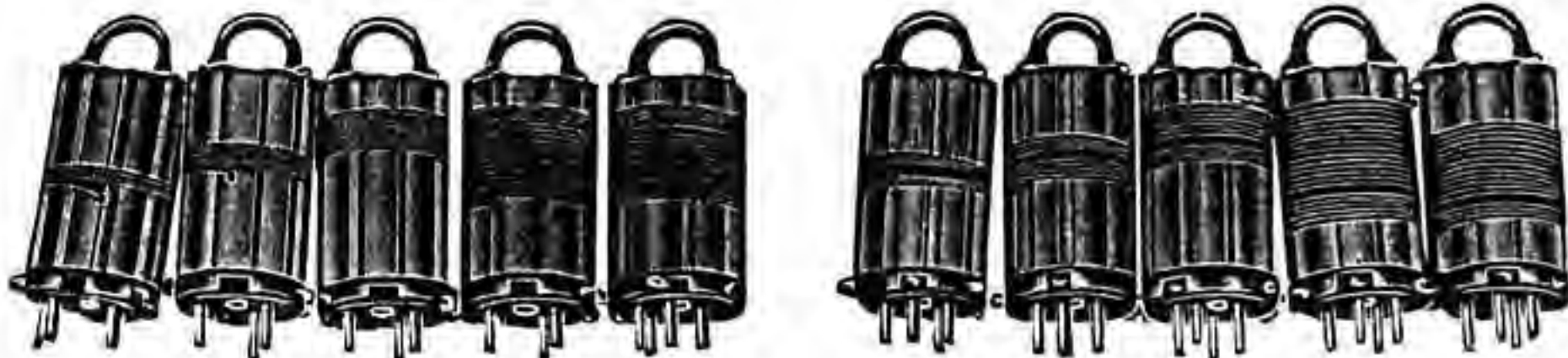
The complete set of plug-in coils for the Super-Wasp. Left, antenna stage coils; right, detector stage coils. Their wavelength range is 14-500 meters.
