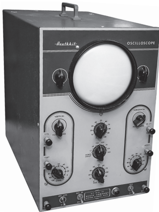
Fig. 11. First electronic Heathkit, the O-1, a 5" oscilloscope showing details of the front panel and controls, July 1947. (Author's collection)
