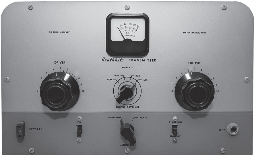
Fig. 19. First all-Heathkit amateur radio transmitter, the AT-1, a 6-band CW transmitter, produced between 1952 and 1956 for $29.50. (Author's collection)
