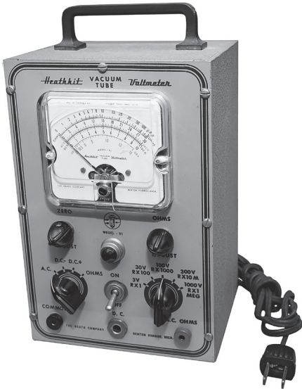
Fig. 14. The author's V-1 VTVM, Type I with five ranges. (Author's collection)
