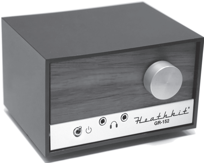
Fig. 25. Heathkit Explorer Jr. GR-152 TRF AM radio receiver kit (solder-type), purchased in 2018 from Heath. (Author's collection)
