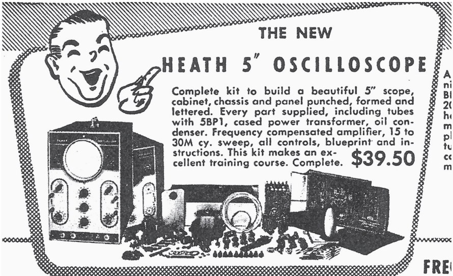
Fig. 10. Ad showing the Heathkit O-1 oscilloscope and parts. ( Radio News , Nov. 1947, p. 102)
