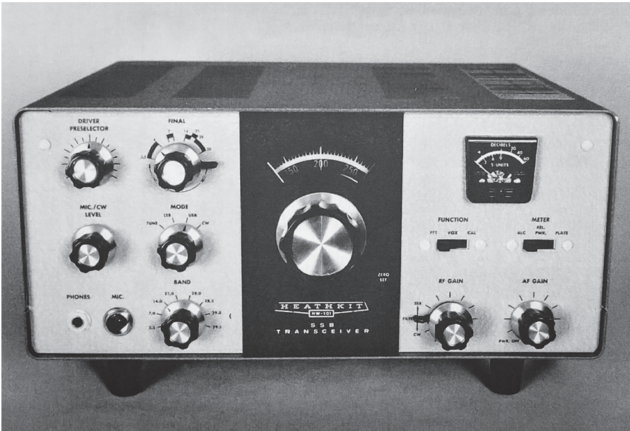
Fig. A-1. HW-101 5-Band Transceiver manufactured between 1970 and 1983, priced at $399.95. (Penson, Heathkit: A Guide to the Amateur Radio Products , 2003, p. 171)
