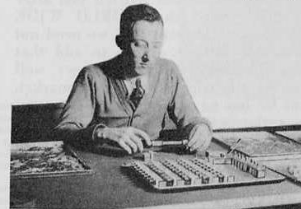
Assembling the small "trimmer" condensers, a part of the special air-tuned I.F. units used in the WORLD WIDE NINE.
