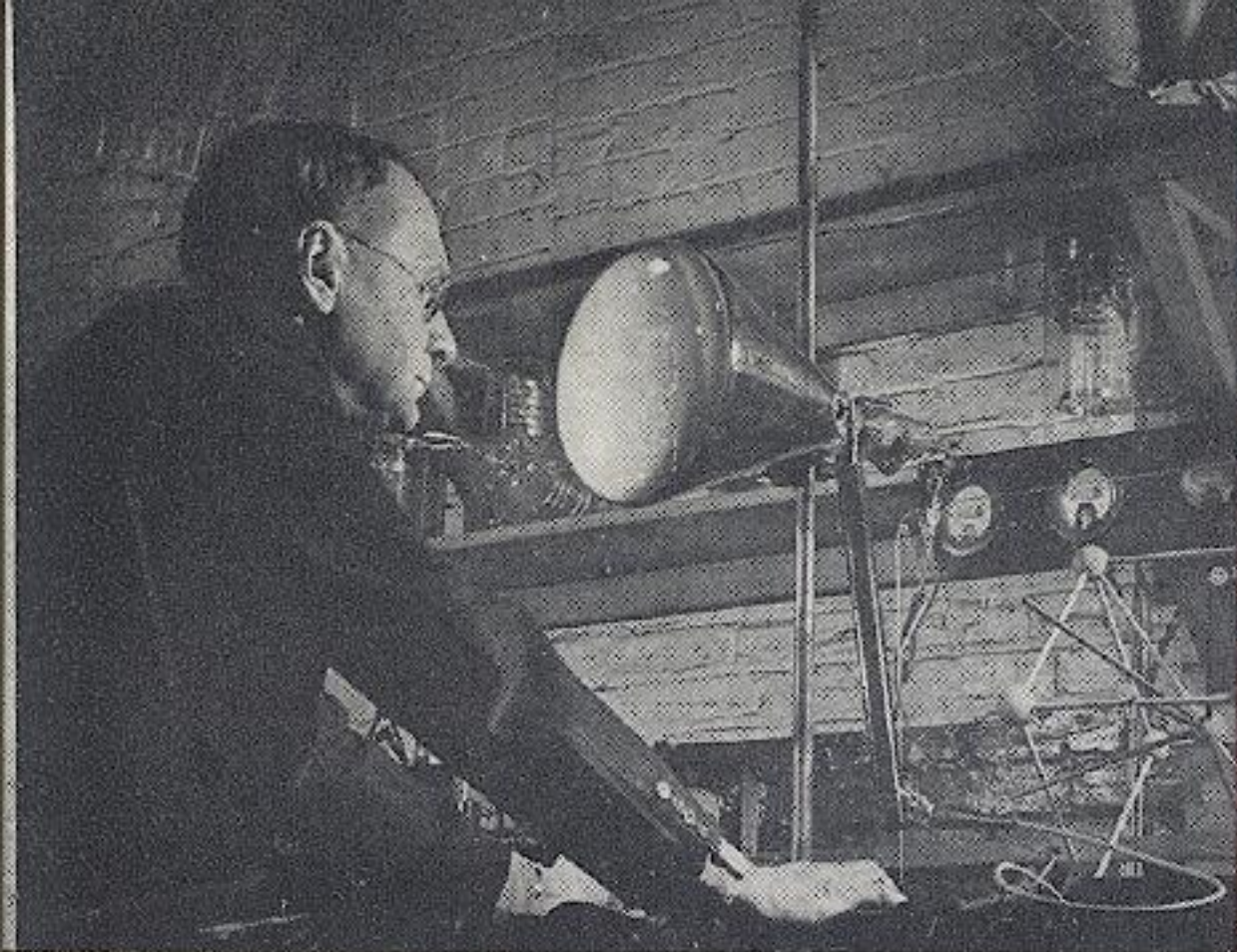
Testing the Kinescope, heart of the television receiver, in the RCA Research Laboratories.
