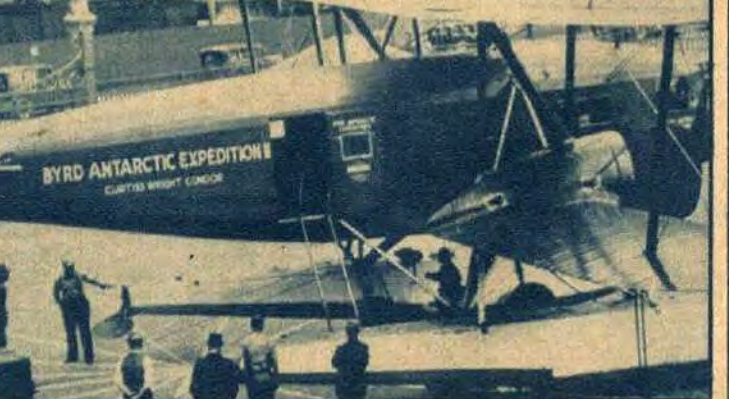
Admiral Byrd, to insure accuracy of his compasses during the three exploratory flights over the South Pole regions, had his navigating instruments checked at the expedition's last stop before setting out for the Bay of Whales. The giant Curtiss-Wright Condor plane, in the center of a circle marked off in degrees, is shown on the docks at Wellington, N. Z.
