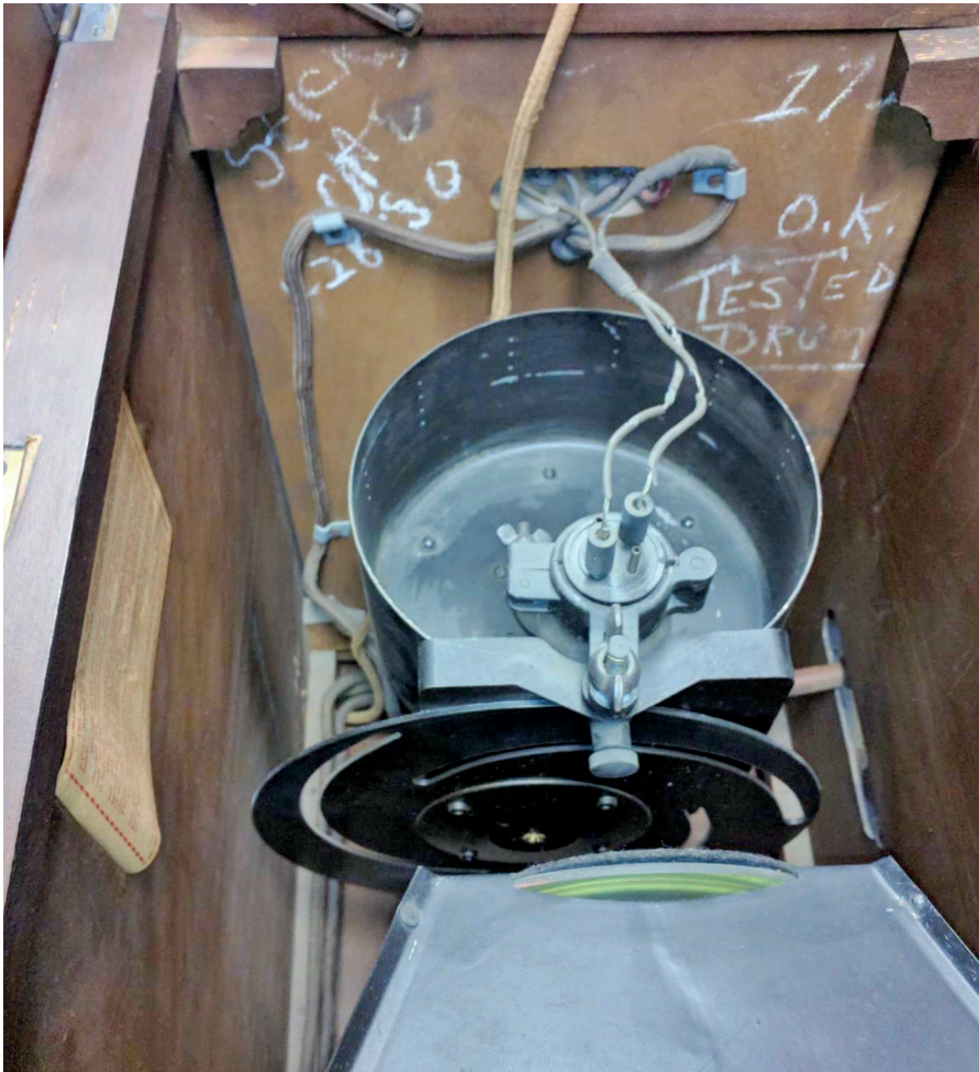
Fig. 3. The interior of the Jenkins Model 201 differs from the other mechanical televisions of its day. The use of a perforated drum to scan the neon tube removed keystone distortion and permitted a narrower cabinet.
