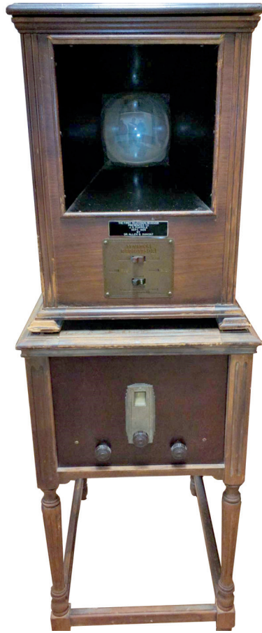
Fig. 1. This Jenkins Model 201 "Televisor" television receiver, which appeared in a TV Guide article in 1971, was owned by Jack Poppele and is now on display in the AWA Museum.
