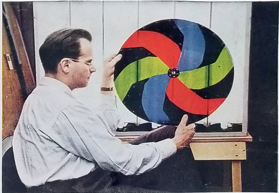
Color disc , held by Inventor Peter C. Goldmark, spins in front of cathode-ray tube. Synchronized with color drum, disc transmits the successive single-color images picked up by camera. Persistence of vision in eyes blends separate color images into integrated full-color picture.
