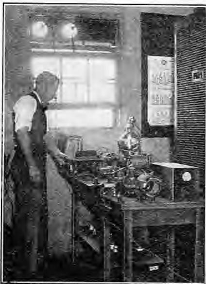
This is the 500-watt transmitter of W2XE, in New York, that makes such a big noise in the ether on 49.02 meters
