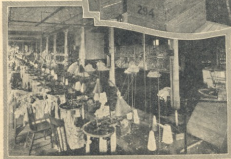
A view of looping machines which join the upper part of the reinforced toe of hosiery to the foot of the hose
