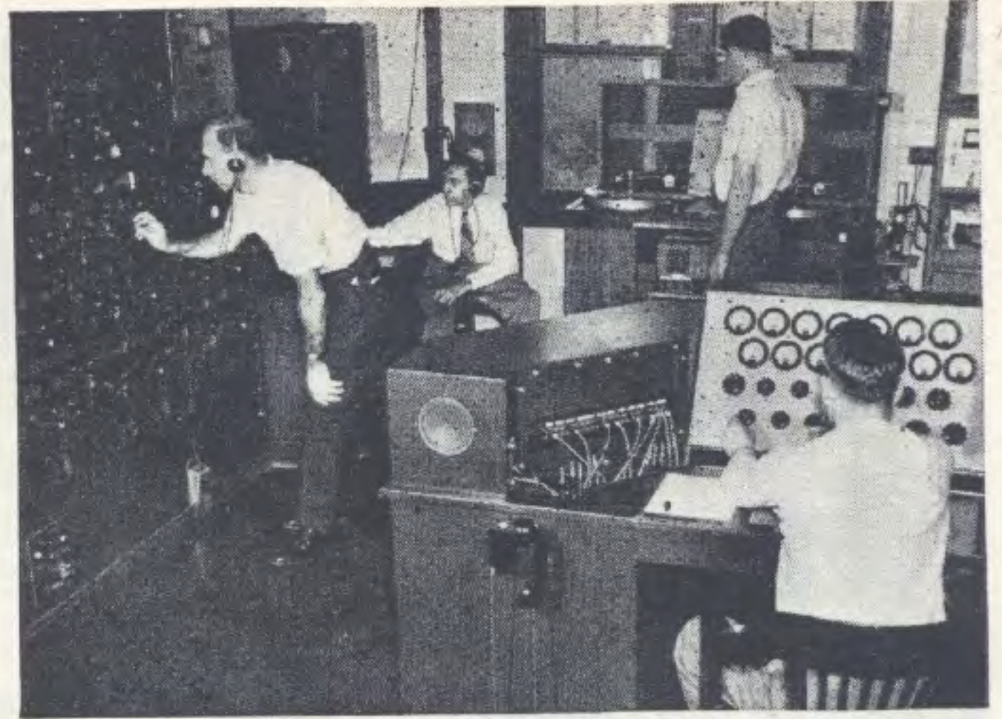
Radio transmissions are picked up by 29 SX-28 receivers and piped through the console (foreground) to the wax cylinder recorders located seven miles from this receiving station.
