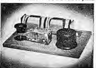
This is the finished job. Notice position of parts. Bracket on this end of batteries does not connect with bracket that goes around batteries.
