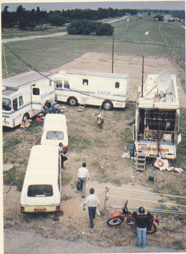
The SABC's outside broadcast vehicles are used to record events on videotape or relay them in direct transmissions.
