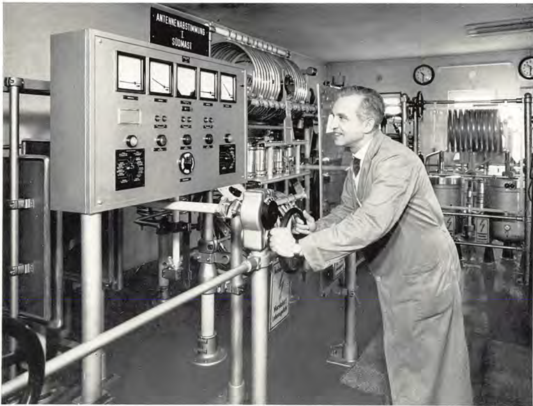
▲ The tuning equipment through which the output of the medium wave transmitters in Berlin are fed into the antennas
