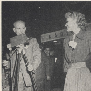
MINIATURE TV camera, designed chiefly for industrial plants, can be carried and operated by one man. The life-size face at right was photographed directly from the TV receiver, linked to the camera by cables.
