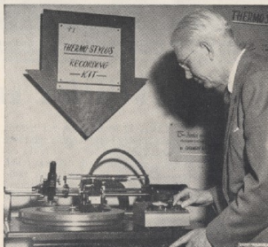
HIGH-FIDELITY noise-free recording is made possible by this machine with a heated stylus as a cutting edge.
