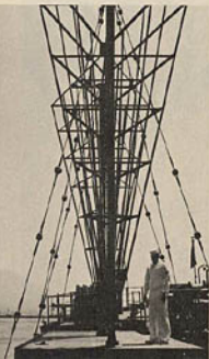
The Coast Guard cutter Courier uses this antenna and both medium and shortwave transmitters to beam Voice of America broadcasts to Soviet Orbit from vessel's berth off Island of Rhodes.
